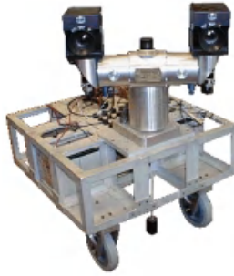
Fig. 1. A typical stereo pan-tilt head, mounted on a mobile robot
